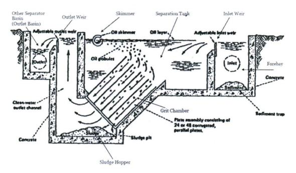
Notably, the definition in Subpart QQQ exactly describes this diagram. All of the components listed in Subpart QQQ (separation tank, forebay, other separation basin, skimmers, weirs, grit chamber, and sludge hopper) are identifiable on the diagram, and they are components of the separators as described by EPA. See Background for Proposed Standards, supra, at 3-30.
