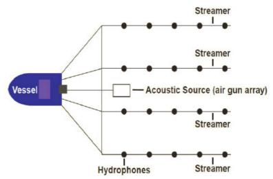
J.A. 20254. If there is a cross-current, the streamers may drift and become offset from the towing direction of the vessel. This phenomenon is known as "feathering." The extent to which the streamers become offset from the towing direction of the vessel is known as the "feather angle." In other words, the streamers, while organized so as to be in parallel with each other, are collectively "offset" at a small angle from the direction of the ship towing the streamers.
