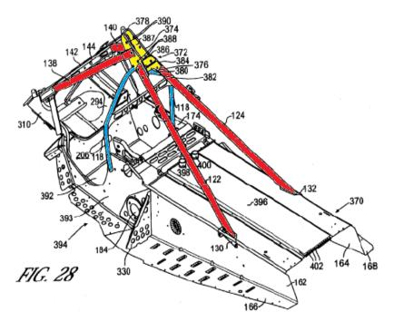
*Id.* Fig. 28 (annotated). The legs and the upper column connect to the steering bracket (374) at the apex of the pyramidal brace assembly (372). *Id.* at col. 12 ll. 46–48.
