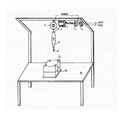
J.A. 297. IBM discloses an electronic torque driver [11] linked to a microcontroller circuit [6]. J.A. 298. IBM states that the microcontroller circuit [6] can "enable/disable the power to the torque driver [11]" and "sense[s] when correct torque is achieved by linking into a hall effect sensor in the driver 11." *Id.* The "controller may be programmed" such that an operator must "wait for the set torque to be achieved on each screw before moving onto the next screw." *Id.*
