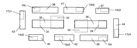
*Id.* at Fig. 3. Local interconnects 38 and 39 correspond to bitlines and are each associated with a single contact region (i.e., regions 16c and 15c). *Id.* at col. 13 ll. 12–14. Local interconnects 43 and 44 correspond to a global wordline are also each associated with a single contact region (i.e., regions 17c1 and 17c4). *Id.* at col. 13 ll. 31–32.
