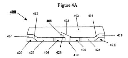
As shown in Figure 4A, the surface mountable opto-electronic device 400 includes an optically transparent body 402, two electrical contacts, 404, 406, and a LED 408. Id. at 4:60–63. The two electrical contacts are mounted in the
