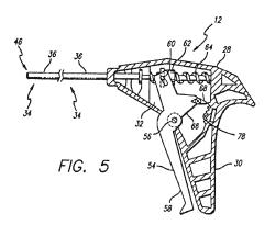
The applicator has a proximal portion (28) having a handle (30) and actuator (32). (Col. 3:21-22, col. 7:65-67) It also has an elongate distal portion (34) for housing fasteners, comprising an outer tube (36) housing an inner rotator (38), a lock clip/indicator (40) and a load spring (42). (Col. 3:19-21, col. 8:7-9) Preferably, a thread form (201) comprising an interlock spring is provided within the outer tube of the distal end, as pictured in fig. 7, below.
