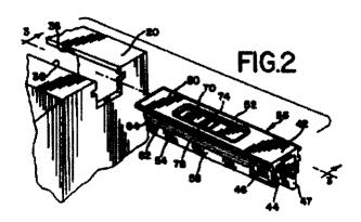
According to the '291 patent, each side wall of the tilt latch has a rail which cooperates with the edges of the housing cover to form a *longitudinal groove* that cooperatively receives the header rails. ('291 Patent, Col. 3, lns. 64-68) The longitudinal groove is the empty space directly above the side wall rail (the yellow structure) and below the housing cover.
