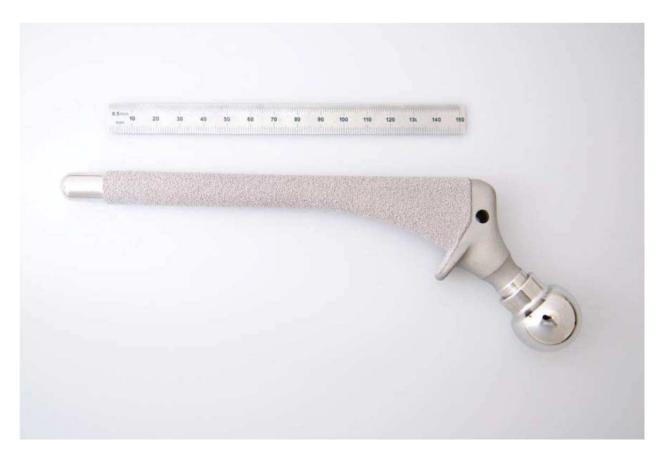
(Kurtz Rep. at 6) (showing sample femoral Head and Stem.) The Head and the Stem fit together to form a junction. (Zimmer Mem. in Supp. of its Mot. for Summ. J. [41], hereinafter "Zimmer MSJ Mem.," 2.) The interior of the Head is a hollow cone that allows the top of the Stem to fit inside it:
