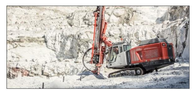
Plaintiff's customers used the equipment for aggregate production. But Defendant's website identifies numerous other uses for its surface drill rigs, including road and railroad construction; demolition; production in large quarries, open pit mines, and construction work sites; and blasthole drilling in mining, quarry, and construction industries.<sup>6</sup>
