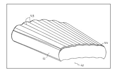
('542 patent, Fig. 4). The main difference between the diagram and the actual product is that that on the actual product the metallic coating is much thinner; it is only a few nanometers thick, far thinner than a human hair. Defendant Sabert Corporation originally produced similar utensils coated on both sides with stainless steel, but changed the product in an attempt to avoid infringement by using a titanium coating and making the plastic substrate opaque.
