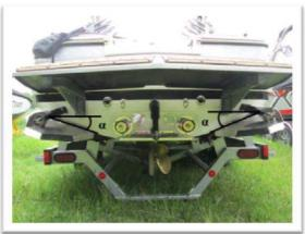
[Doc. 24 p. 10]. When the operator of the boat deploys one side, the boat leans to the non-deployed side [Doc. 26 ¶ 17; Doc. 26-23]. Like with the Surf Tabs, the port wake-shaping device is deployed in order to enhance the starboard surf wake, and the starboard wake-shaping device is deployed in order to enhance the port surf wake [Doc. 26 ¶ 16].
