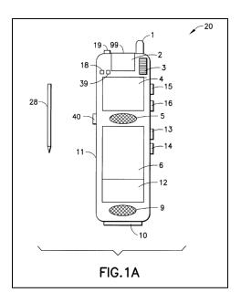
*Id.* at Figure 1A. The specification states that the device includes "a reading head 2, for example a camera or infra-red optical reading head (e.g. laser diode), suitable for capturing data and/or images . . . ." *Id.* at 5:38–40. The specification further states that "[t]he reading head is preferably interchangeable through the use of a clip-on enclosure 99, to allow the use of different types of reading heads." *Id.* at 5:42–44. The specification adds that "[a]n adjustment thumbwheel 3,
