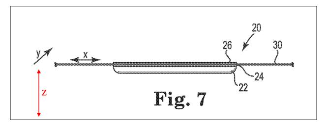
intermediate layer along the y axis. The efficiency may be increased by also moving the wire in the x axis in a reciprocating or continuous motion. *Id.* at col.6 ll.32–42.
