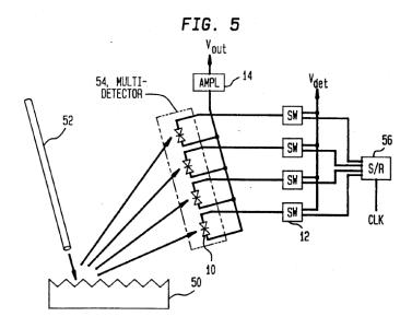
Chang '527 also discloses that "[e]ach switch 12 selectively applies a bias voltage supplied by a source of voltage  $V_{det}$  to the selected detector 10. All photo-detectors 10 supply their photocurrents to a single amplifier 14, which outputs an amplified signal  $V_{out}$ ." Chang '527 at 3:31-35.
