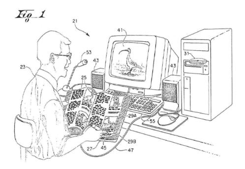
WILLIAMS, FIG. 1. In addition, the Examiner took the audio signal generator claimed by the patent applicant to be similar to the sum of the components of bar code reader 57, disk 31, computer system 33 and audio speakers 43. *See* WILLIAMS AT 3:29-30; 3:33; 3:43; and 5:13.
