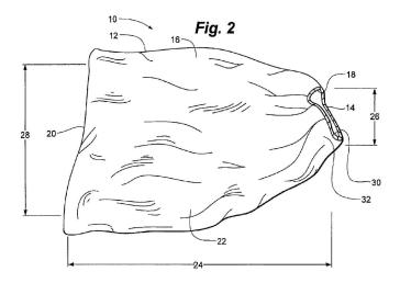
As Figure 2 demonstrates, the center portion is what gives the duct cover length, allowing it to extend over part of the duct's exterior. The center portion works in conjunction with the elastic to hold the duct cover onto the duct.
