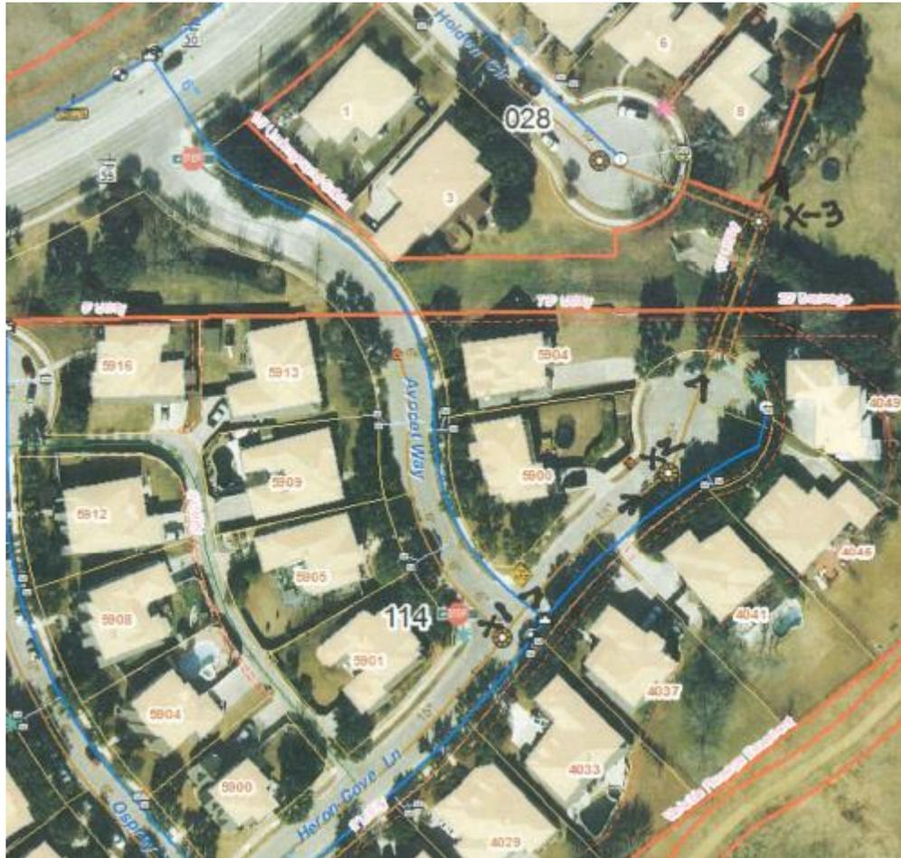
Maintained by the City, the sewer main is “entirely gravity flow,” flowing downstream in a northeasterly direction, as denoted by the arrows in the image along its route. Residential properties tie in to the sewer main via lateral lines. The Ryghs’ residence is adjacent to the manhole located at the intersection of Heron Cove Lane and Avocet Way (X-1).
