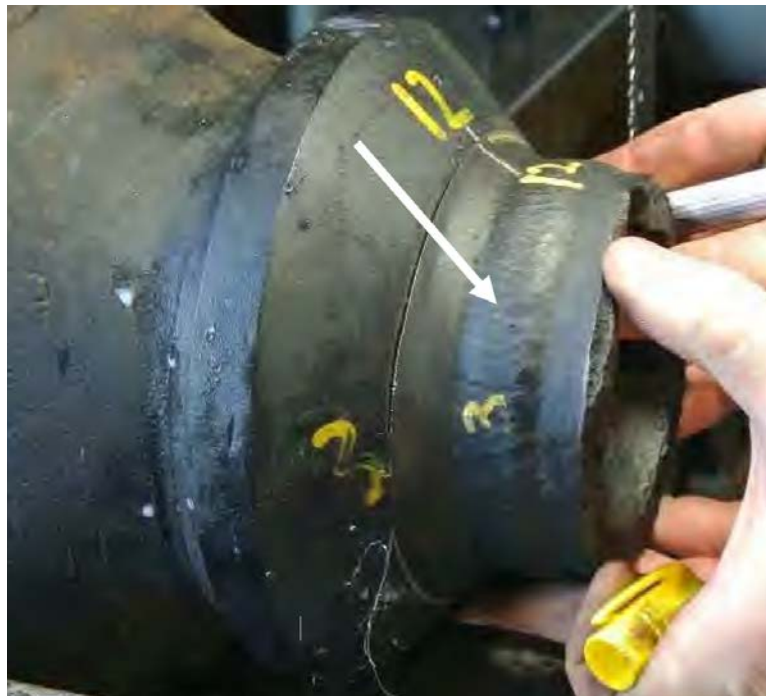
Close-up image of FV-241 after it fractured. The arrow points to the weld that connected FV-241's valve body to its welded-on flanges.
