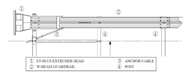
A diagram of the ET-Plus system prepared by TTI and Trinity.
