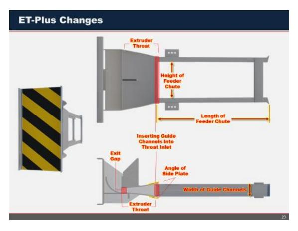
A diagram prepared by Harman listing the purported changes to the ET-Plus terminal head in 2005.
