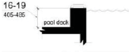
Fig. 75 Transfer Wall Height
