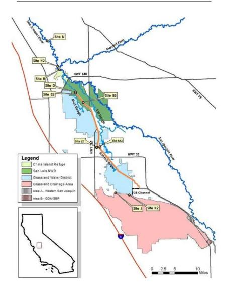
The Project includes the San Luis Drain (the Drain), labeled on the map above, which is designed to collect and convey contaminated groundwater from lands adjacent to and upstream of the Drain to Mud Slough. As both parties
