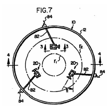
In Figure 7, impellers or pumps 20 that are placed within the claimed radii of  $r_1$  and  $r_2$  create the substantial helical flow as shown in Figures 5 and 6.
