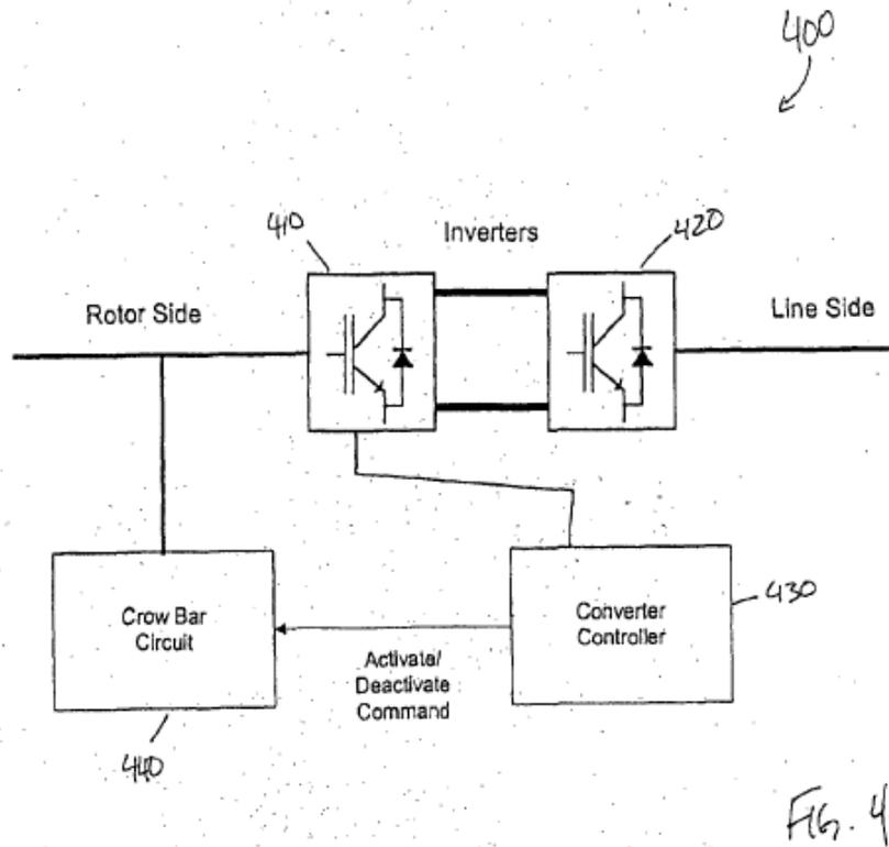
Figure 4 shows back-to-back inverters as part of the power converter; the inverters receive power as needed during a low voltage event “to keep the wind turbine generator connected to and synchronized with the power grid.” ’985 patent, col.6 ll.27-29. The specification describes the connections and functions of the components, including the following:
