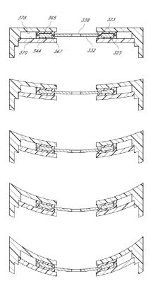
J.A. 4816. At the top of the diagram is an embodiment of the '379 patent. By gradually curving this embodiment, the expert arrived at a hypothetical instrument seal assembly that he claims is similar to the Covidien Trocars' gimbal seal assembly. According to the expert, this demonstrates that the '379 patent instrument seal assembly and the gimbal seal perform the same function in the same way to achieve the same result.
