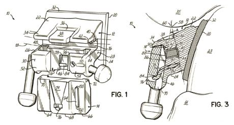
Slot 16—formed by base surface 40 and opposite sides 42 and 44—holds archwire 18. Slide 14 slides up along support surface 46 to cross the slot and then lodge against ledge surface 92 of ledge 90. The slide moves along plane 60 (defined by the support surface), which forms Angle A with plane 58 (defined by the base surface). The angle allows the slide to avoid gum 61.
