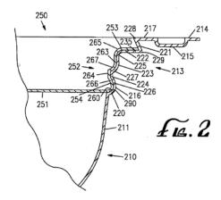
As depicted in Urciuoli Figure 2, the lid **250** nests within the edge or lip **222** of the container portion **210**. The frangible breakpoint **235** in Urciuoli is located in this lip section that lies around the container. To open the container of Urciuoli, a user applies pressure to a handle **215** on the container portion, breaks the frangible section, and lifts the lid portion out from its nesting position in the container portion.
