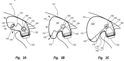
Under normal operation, as the airbag cushion inflates, the cord pulls taut and closes the vent. When the occupant is out of position, the cord remains slack and the closeable vent remains open, permitting rapid release of excess gas through the closeable vent.
