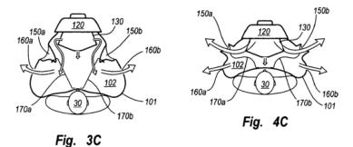
In Figure 3C, the occupant (30) is in proper position, allowing the cords (150a, 150b) to fully extend and close the closeable vents (160a, 160b). In Figure 4C, the occu-
