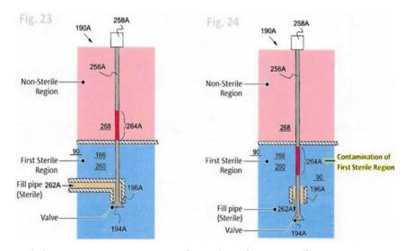
Decision at 331 (annotated). As shown, when actuator 258A displaces valve stem 256A in a downward direction, valve 194A is removed from nozzle 196A, allowing product 262A to flow into a bottle. '591 patent at 14:1-16. When this happens, portion 264A of the valve stem goes from nonsterile region 268 into the first sterile region 260, potentially contaminating the first sterile region. Id. at 14:16-23.
