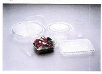
NatureWorks® PLA Packaging is made from corn and is a clear, nature-based alternative to traditional fossil fuel derived food containers. The natural package can be composted in industrial facilities. The carbon and other elements in natural plant sugars are used to make plastic, called polylactide (PLA), through a simple process of fermentation, separation, and polymerization. NatureWorks(tm) PLA is helping retailers worldwide draw attention to and drive sales for their fresh food
