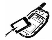
**e.** Replace the battery and make sure connectors from battery match up with the phone.
