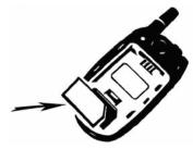
**d.** Line up beveled edge of Smartchip with slot in phone.
