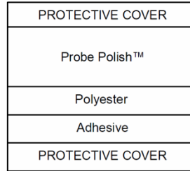
Figure 2: Probe Polish Cross Section
