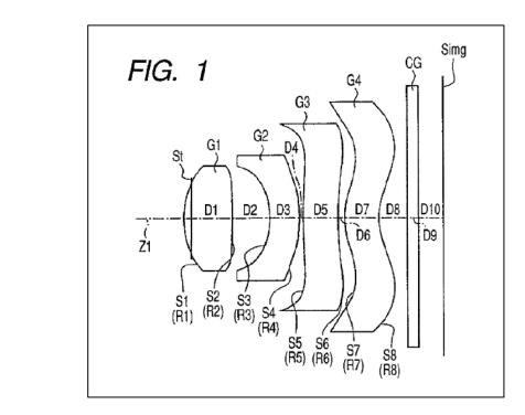
Id. at fig.1. The configuration has four lenses—G1, G2, G3, and G4—labeled in increasing
