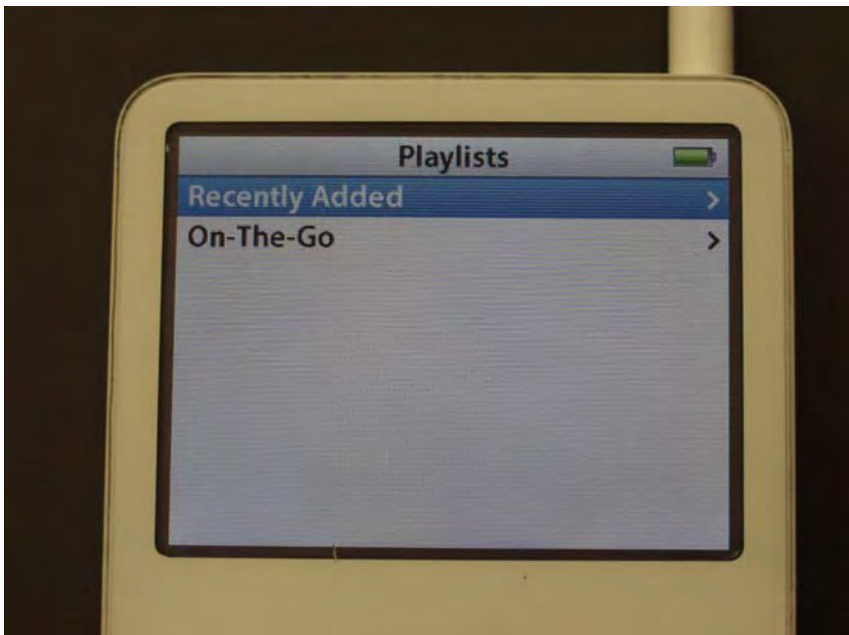
Figure 27. iPod video showing that the “On The Go” (without dashes between the words) playlist is not displayed.
