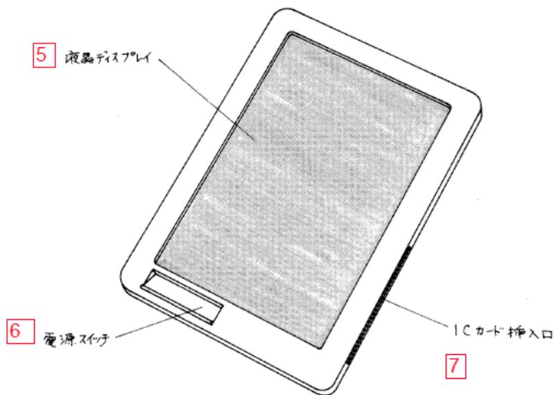
1-perspective view, 2-reference front surface view showing electric current conditions, 3-cross-section along A-A omitting internal structure, 4-drawing showing outline of operating part, 5-liquid crystal display, 6-current switch, 7-IC card inlet
