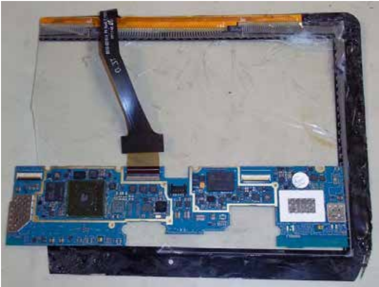
Figure. Camera image of the Galaxy Tab 10.1 touch screen, connective flexboard, and circuit board. See Exhibit C-64.
