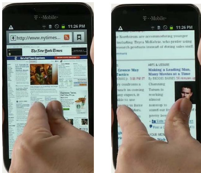
17 Fig. 15: Galaxy S II Browser detecting and responding to a de-pinch gesture
