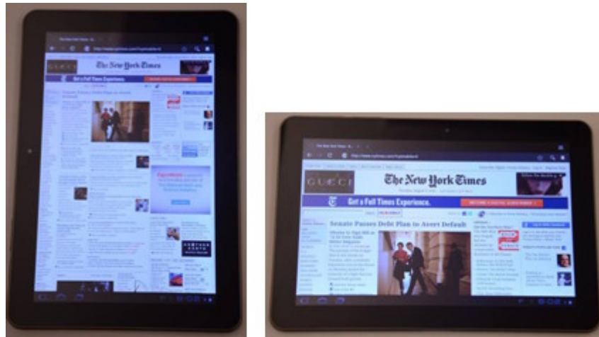
12 Fig. 12: Galaxy Tab 10.1 Browser scaling the document width to fit within the display width 13 independent of the document length
