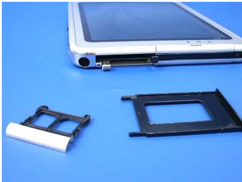
Plastic cards like these are used to hide the PCMCIA and CompactFlash bays when not in used.
