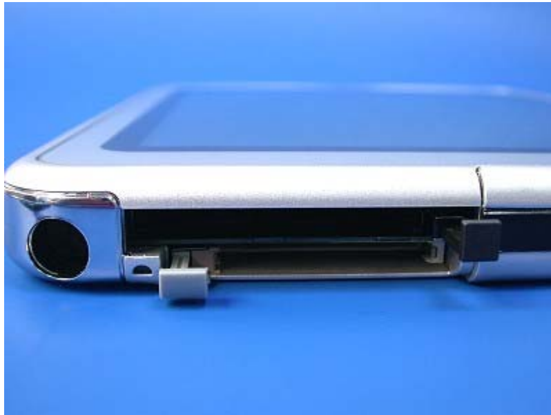
The TC1000 supports a single Type II PCMCIA card, and a CompactFlash slot.
