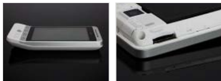
The right side of our Hero is bare, but a microSD slot hides under the armor
