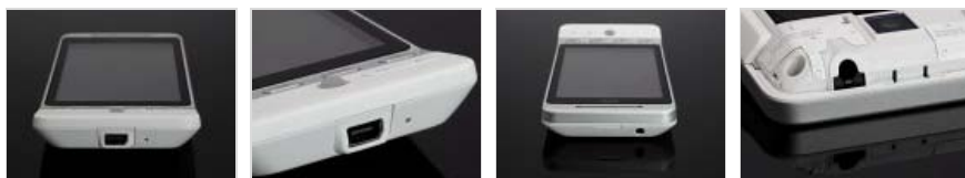
The miniUSB port on the bottom and the 3.5mm audio jack on the top
