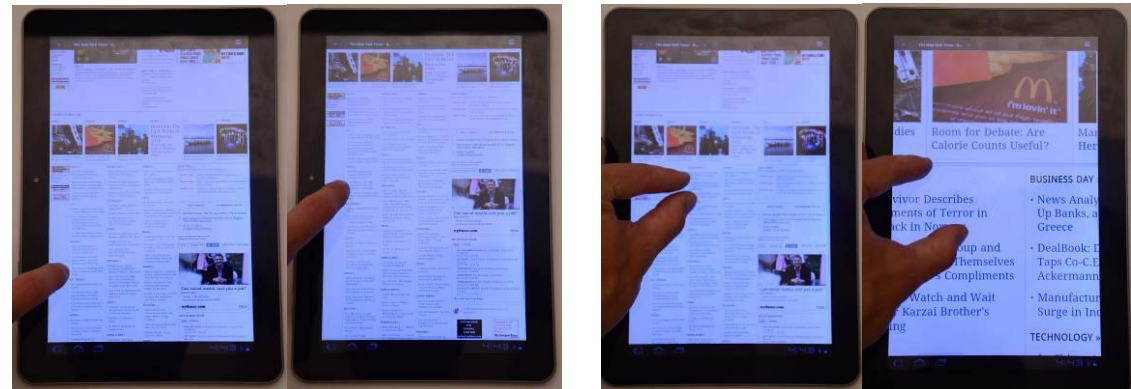
(Screenshots of the Samsung Galaxy Tab 10.1 scrolling in response to a single input point applied to the touch-sensitive display and scaling in response to two or more input points applied to the touch-sensitive display.)
