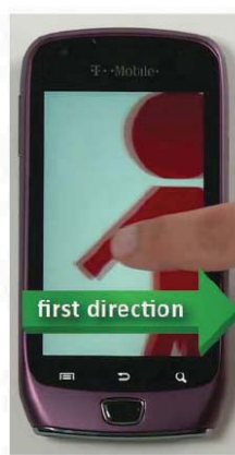
Figure 2: Displaying “second portion” by moving in first direction in response to finger movement
