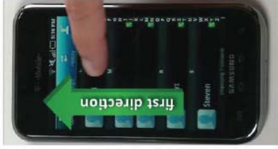
Figure 34: Displaying “second portion” by moving in first direction in response to finger movement
