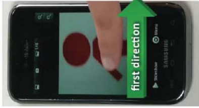
Figure 10: Displaying "second portion" by moving in first direction in response to finger movement
