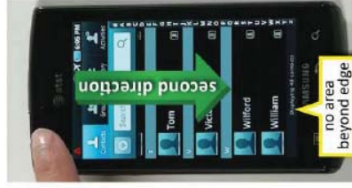
Figure 32: When finger is lifted, document is moved in second direction to display "fourth portion" with no "area beyond edge"
