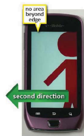
Figure 4: When finger is lifted, document is moved in second direction to display “fourth portion” with no “area beyond edge”
