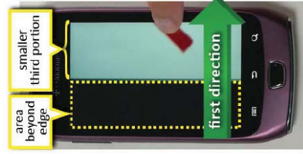
Figure 3: Displaying "area beyond edge" and smaller "third portion" while moving in first direction
