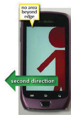
Figure 4: When finger is lifted, document is moved in second direction to display “fourth portion” with no “area beyond edge”
