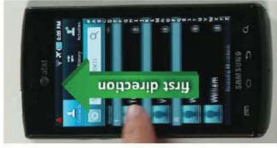
Figure 30: Displaying "second portion" by moving in first direction in response to finger movement
