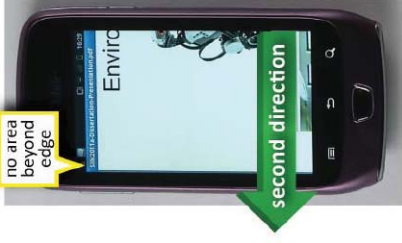
Figure 24: When finger is lifted, document is moved in second direction to display "fourth portion" with no "area beyond edge"
