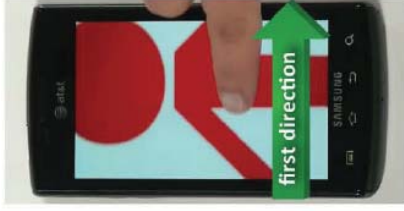
Figure 6: Displaying "second portion" by moving in first direction in response to finger movement
