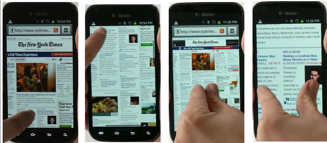
(Screenshots of the Samsung Galaxy S2 scrolling in response to a single input point applied to the touch-sensitive display and scaling in response to two or more input points applied to the touch-sensitive display.)
