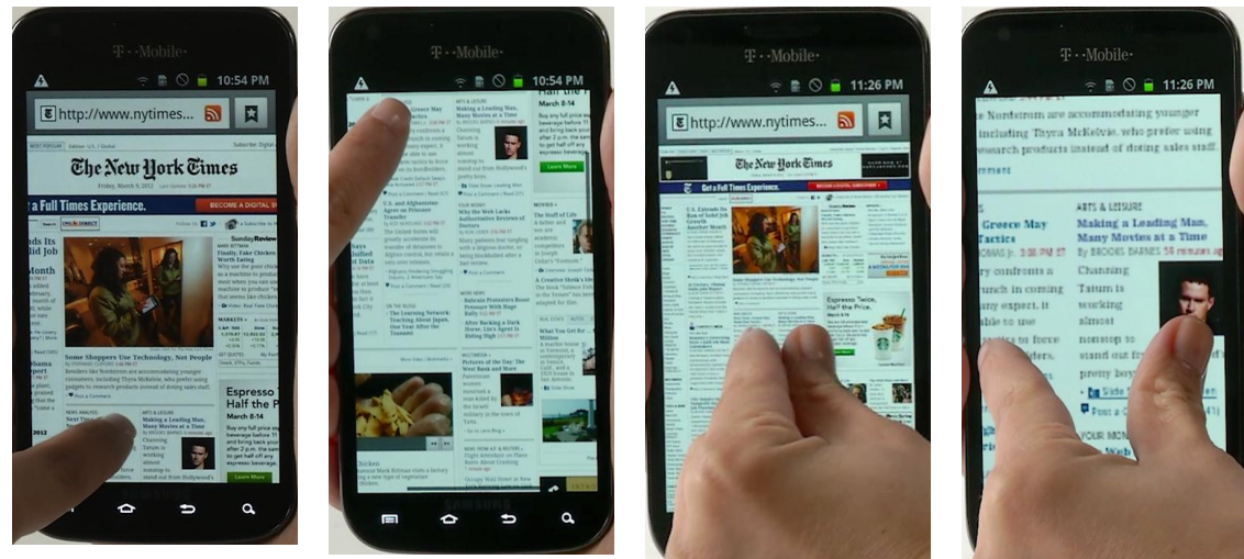
(Screenshots of the Samsung Galaxy S2 scrolling in response to a single input point applied to the touch-sensitive display and scaling in response to two or more input points applied to the touch-sensitive display.)
