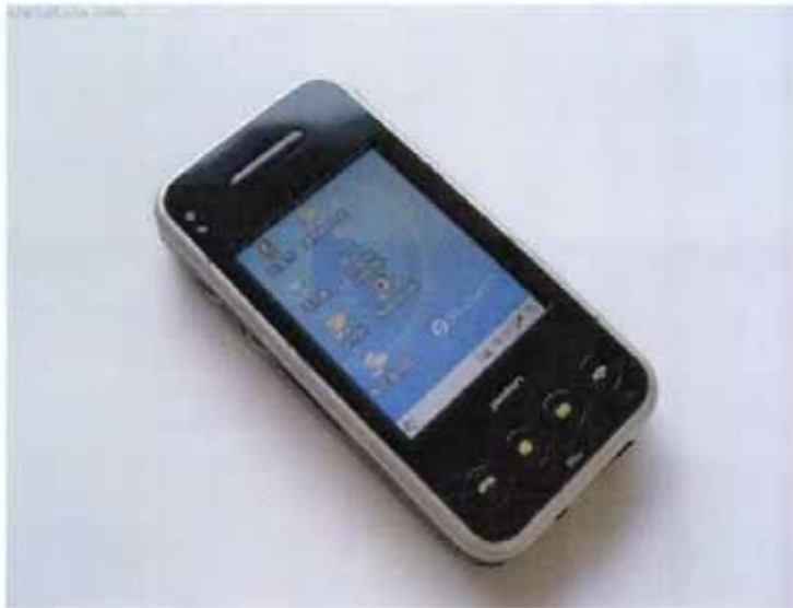
Photoshot of a Korea's gadget. Available in Korea only, Pidion BM-200 is small but has integrated WiFi, bluetooth and running windows CE5.0. The SD card slot is just nice for the 2 megapixel camera. More photos at gizshuforum.com
