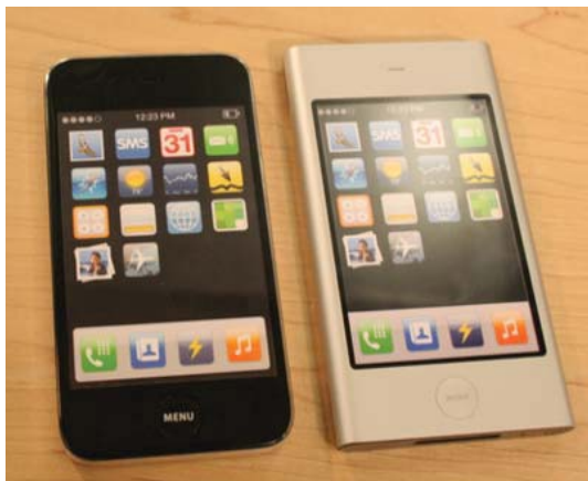
Apple iPhone design mockups (the “Sony style design” is on the left)
