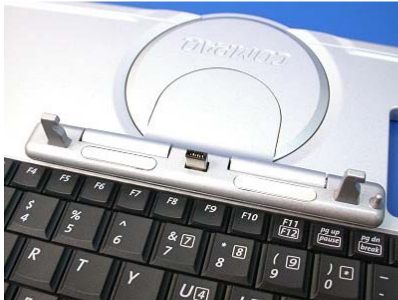
The port that connects the main unit of the TC1000 to the keyboard attachment.
