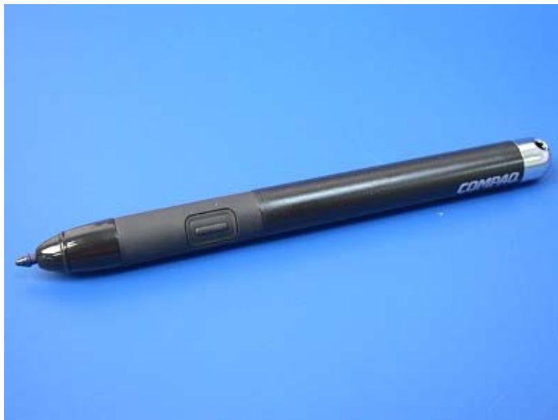
The Compaq Tablet PC comes with a pretty thick but comfortable magnetic pen that sports a pressure sensitive tip.
