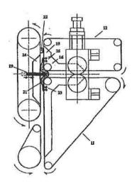
The Fameccanica reference differs from the '187 patent in two major respects. First, Fameccanica does not disclose vacuum rolls; it discloses vacuum conveyors. Second, Fameccanica does not disclose plates that separate the leading and trailing halves of the training pant while the pant is folded at the crotch region.
