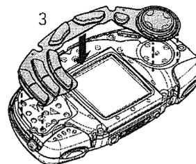
4. To replace the front cover, first place the catches on the lower part of the cover into the corresponding holes in the phone (4) and then gently press the cover into place (5).
