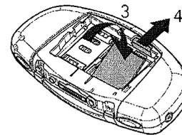
4. When you have secured the card in place, replace the battery and then replace the cover by sliding it back into place. See the step 5 in Installing the SIM card and the battery on page 29.
