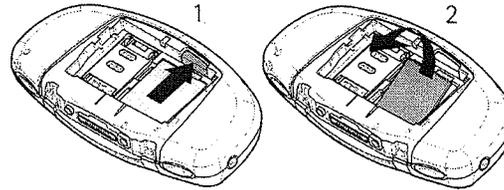
To install the memory card, gently press the memory card into its place (3) while pressing and holding the memory card release button (4). Make sure that the gold contacts of the card are facing down.
