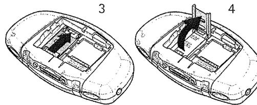
3. Insert the SIM card into the SIM card holder (5). Make sure that the SIM card is properly inserted and that the bevelled corner of the card is pointing upwards and the golden contact area of the card is facing the connectors on the phone.
