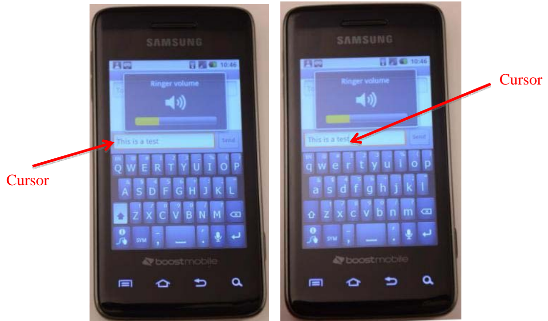
(Screenshot of the Ringer volume window displayed independently of the cursor position.)
