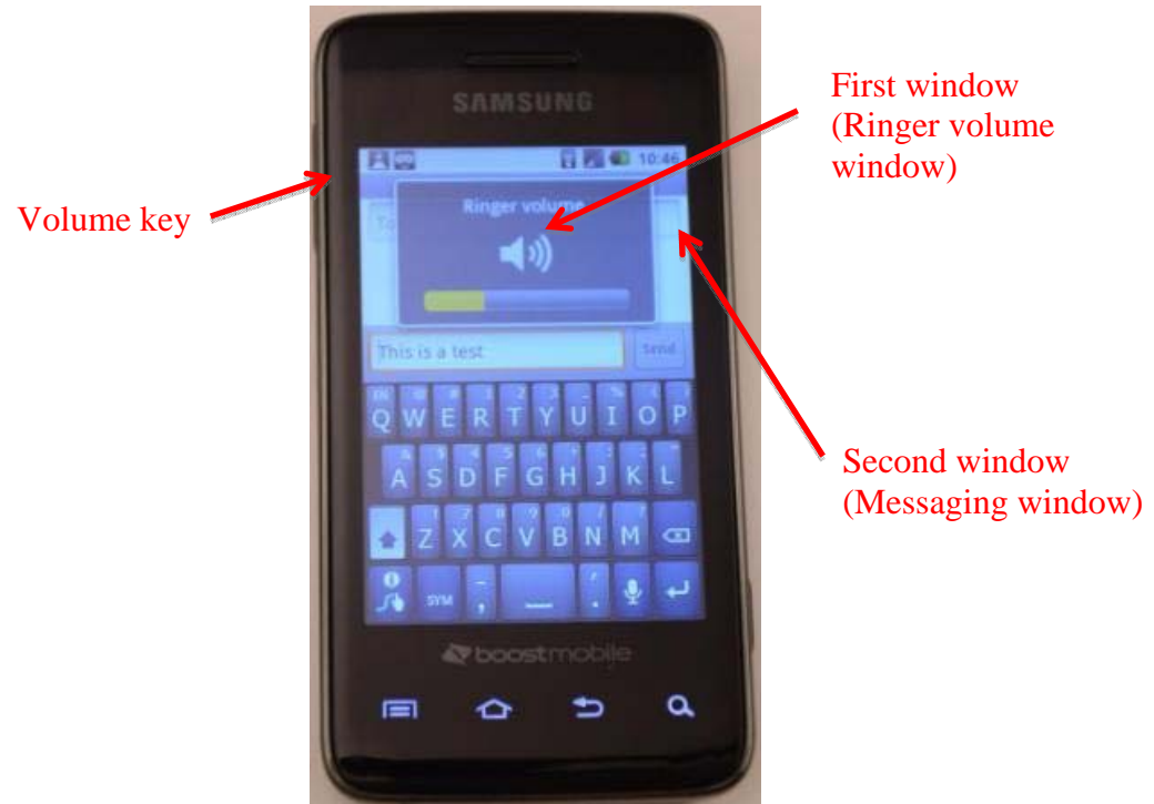
(Front view of the Samsung device showing the Ringer volume window and the Messaging window displayed concurrently.)
