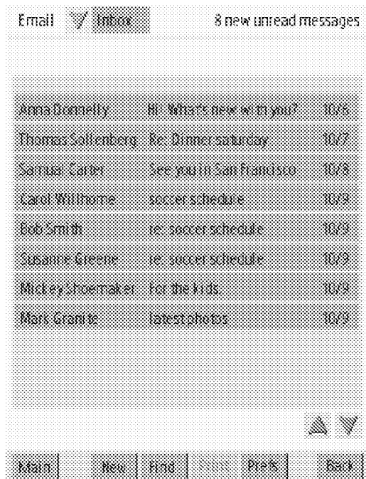
Figure 3: A sample of some of the widgets from the Touchable look and feel in the context of an email application, scaled down to 50% and rotated to vertical. Notice the modified button shape and placement of the scroll buttons.
